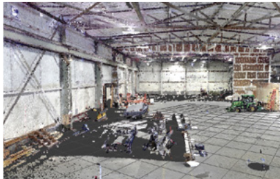
02 "point cloud" (*.rcp) file
