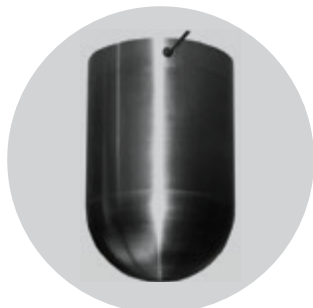
EN 12572-2 Impactor Test mass: 30 kg Object diam.: 150 mm Drop height: 2.2 m
